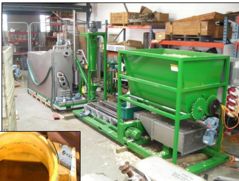
Above: Ernslaw's one tonne per day fast pyrolysis plant developed by AES Ltd,
