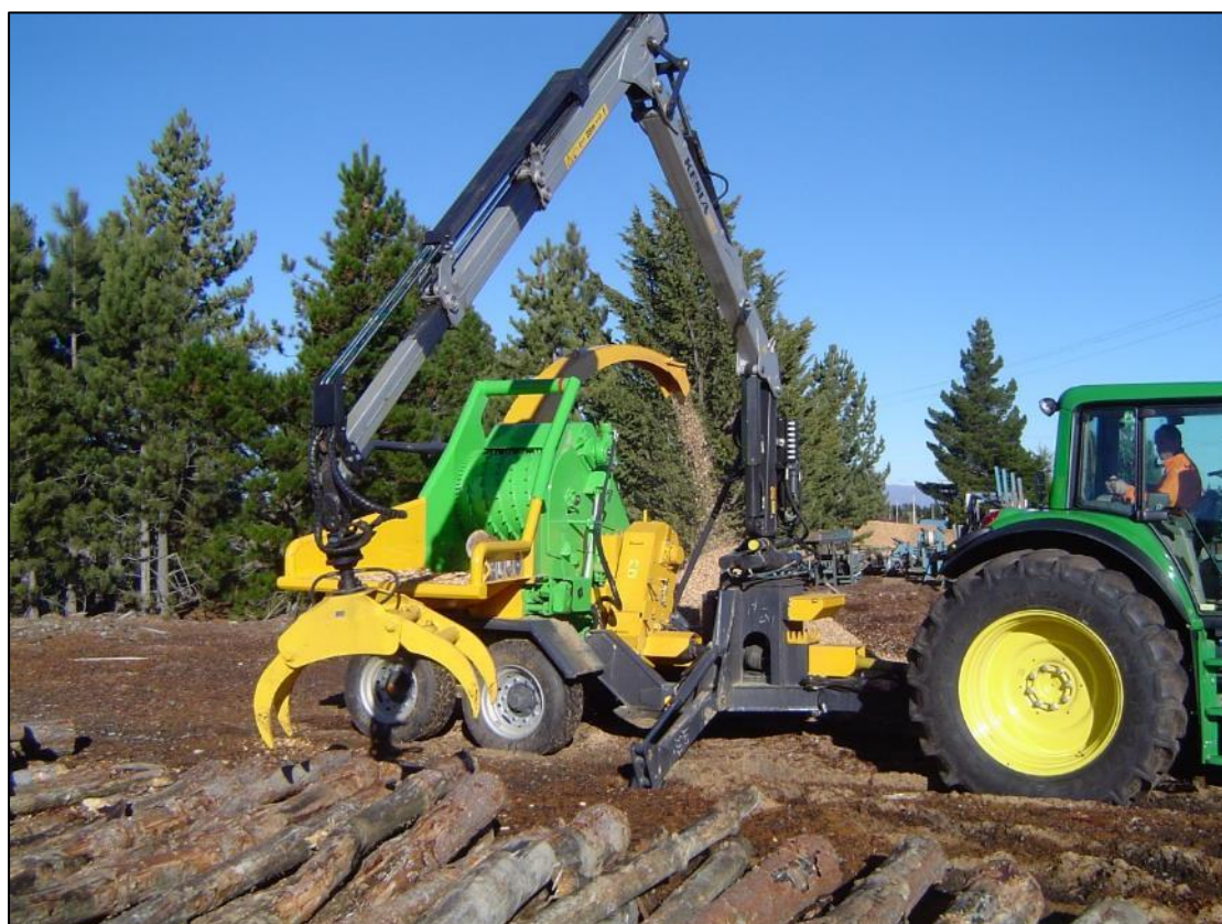
Trials of Ernslaw Bioenergy’s new drum chipper capable of chipping logs of up to 800 mm diameter, 2008 at Naseby Forest in the Maniototo
